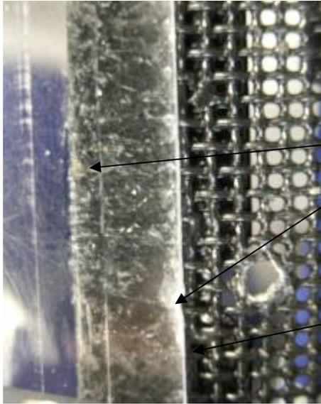
Deep deformations and scratch marks in visor sides.
