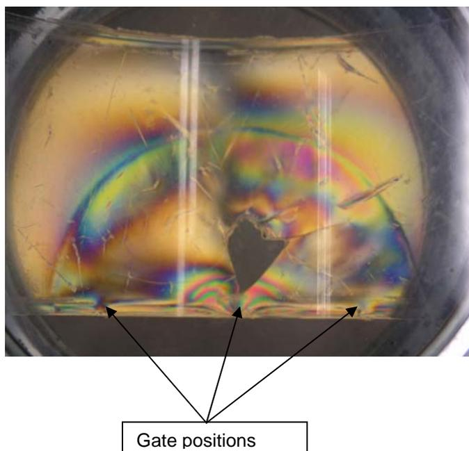
It was then checked if a coating was present on both outside and inside surfaces by means of an ATR/FTIR evaluation. By means of this technique it could be concluded that no coating was present and material of the visor is polycarbonate.
